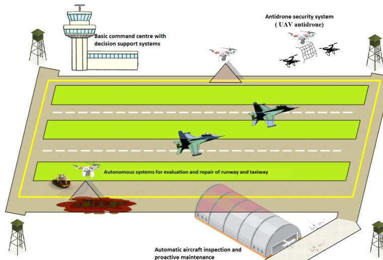
FIG. 2 Use of autonomous systems within the concept of intelligent air base [11]
