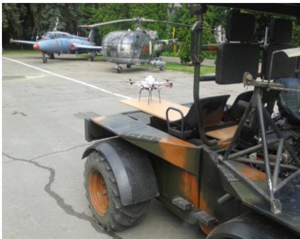
Fig. 4 DAC 2.65 used as an UAV Forward Reconnaissance Mobile Cell (temporary launching platform)
