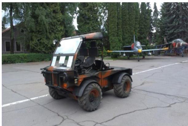
Fig. 2 The light off-road articulated prototype vehicle, DAC 2.65 FAEG
