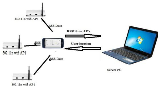
Fig. 3. Framework of indoor positioning system
