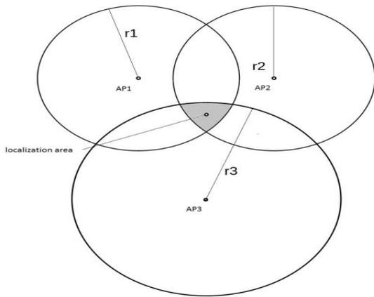
Fig. 1. Indoor localization area provided by trilateration approach
