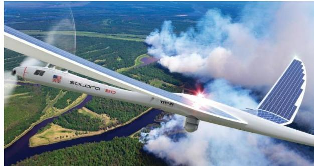
FIG. 1. A TitanAerospace's Solara 50 UAV
