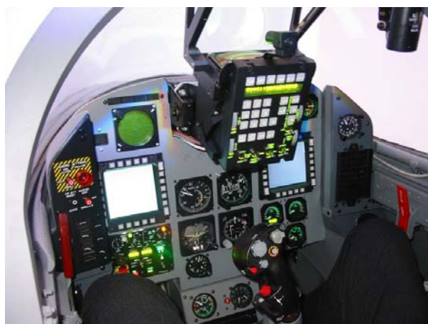
Fig. 4 The cockpit of L-159 with multifunction displays
