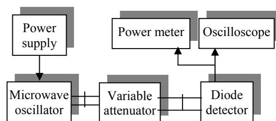
Fig. 2 Measurement setup for microwave field attenuation
