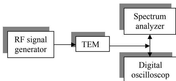
Fig. 1 Measurement setup for the 10 MHz ÷ 1000 MHz frequency interval
