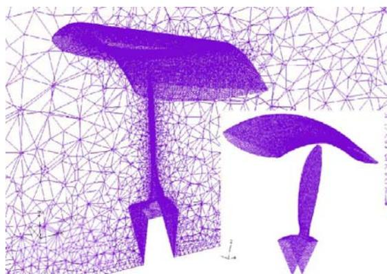
Fig. 2 Unstructured grid – 524 000 tetrahedral cells
