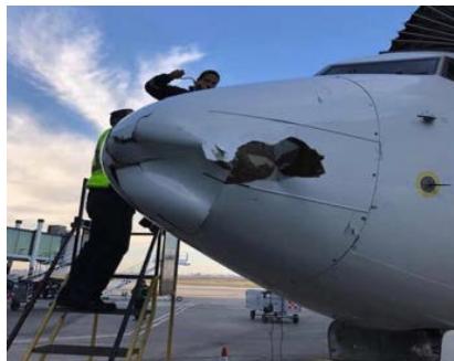
FIG. 6 Mid-air collision with a drone damaged aircraft's nose
