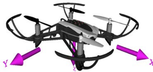
FIG. 4 Position of the three axis for the quadcopter’s movement
