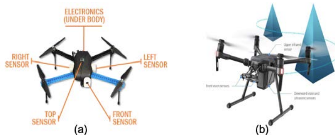
FIG. 2 (a) Position of sensor on a drone, (b) Flight pattern of a drone.
