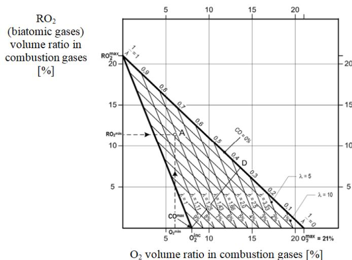
FIG. 1 Oswald diagram (combustion triangle), [2].
