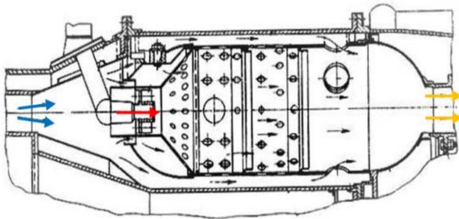
FIG. 2 The combustor. Mix gases circuit, [7].
