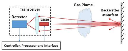
FIG. 3. The operation of the Remote Methane Leak Detector used in [41]
