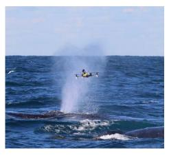
FIG. 2. UAV collecting a sample of whale blow [23]
