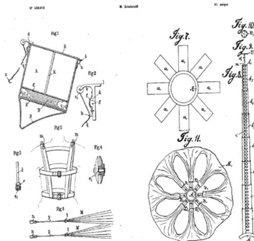
**FIG. 13** Safety device for automatous parachute - Kotelnicoff Gleb - This invention consists of a safety device where the parachute is closed and at the moment of pulling up the parachute is thrown out [23]
