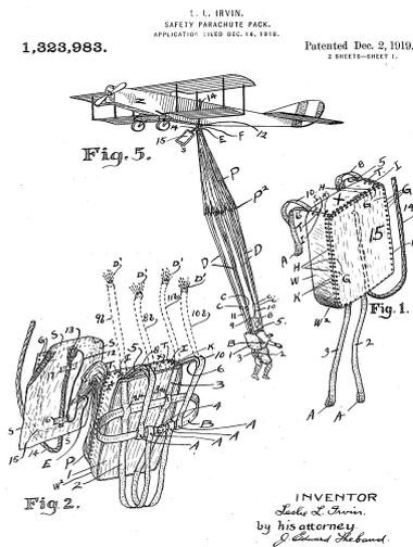
**FIG. 9** Safety parachute-pack – Leslie L. Irvin -This invention relates to safety parachute packs, particularly to that kind which includes the systematically packed parachute and connections in a neat sack. [19]
