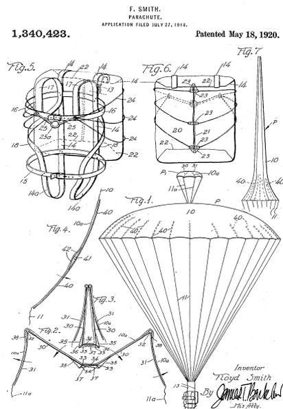
**FIG. 11** Parachute – Smith Floyd - This invention provides a dependable means for causing the straightening out and opening of the parachute under all conditions, including certain conditions under which the present type of parachute is totally inoperative or deficient in operation [21]
