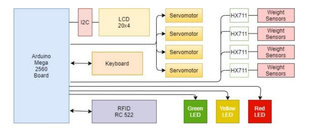
FIG. 3 Electronic diagram of the circuit
