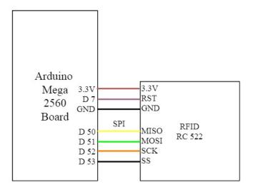
FIG. 7 Block diagram for RFID
