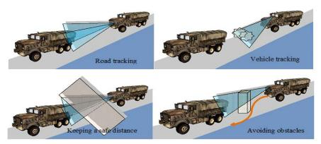
FIG. 4 CAST system capabilities [16]
