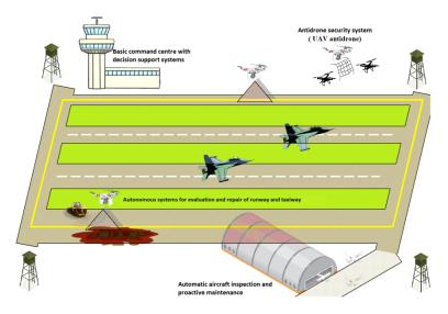
FIG. 2 Use of autonomous systems within the concept of intelligent air base [11]
