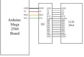
FIG. 6 Block diagram for LCD
