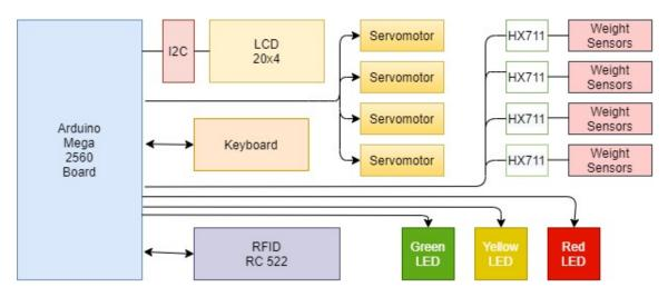
FIG. 1 Electronic circuit diagram
