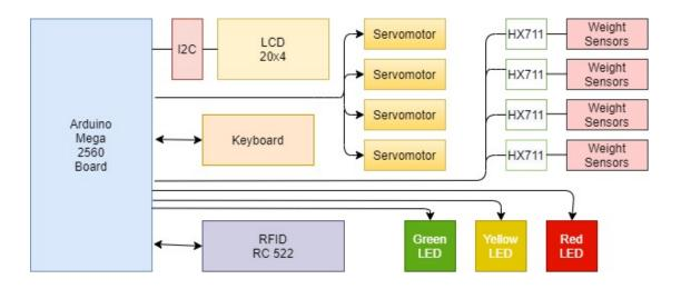
FIG. 3 Electronic diagram of the circuit
