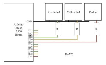
FIG. 8 Block diagram for LEDs
