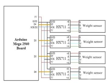
FIG. 4 Block diagram of the weight sensor
