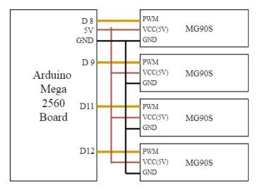
FIG. 5 Block diagram of servo motors
