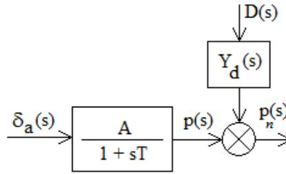
FIG. 3. Block diagram of the SISO UAV model.
