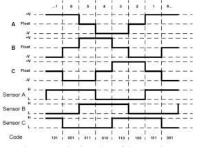
Fig. 5 - Conduction Time of the Transistors
