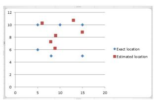
Fig. 6. Positioning accuracy around 2-2.5 m
