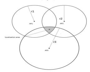
Fig. 1. Indoor localization area provided by trilateration approach
