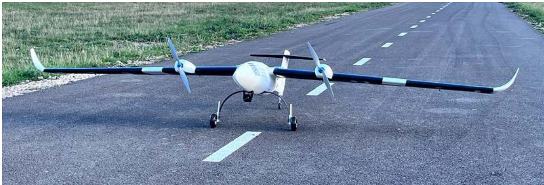
FIG. 1 Fixed-wing twin-engine aircraft made from 3D printed composite materials [10]
