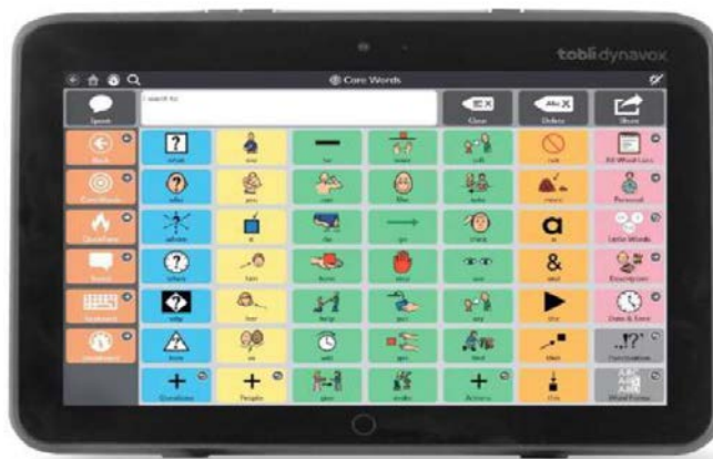
FIG. 4 High-tech specialized speech generation device I-110 (Tobii Dynavox) with touch screen.
