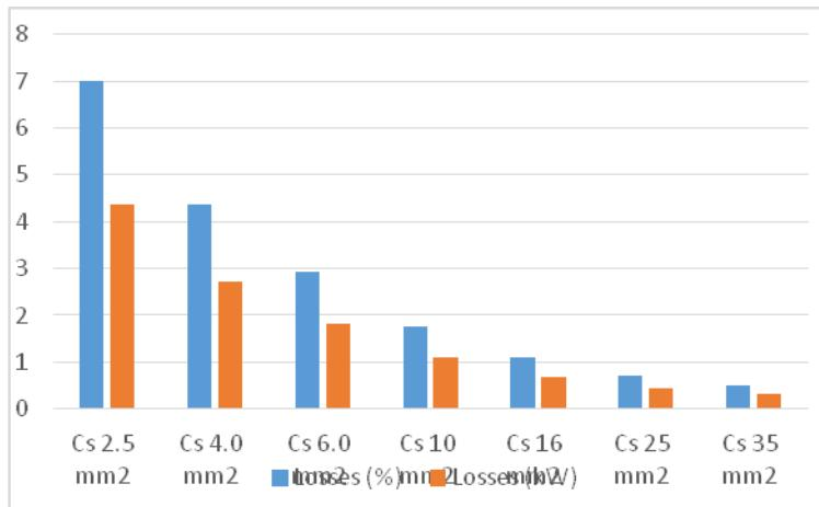
**Graph 2.** Energy losses according to solar wire cross section (for a 62.5 kW solar installation)
