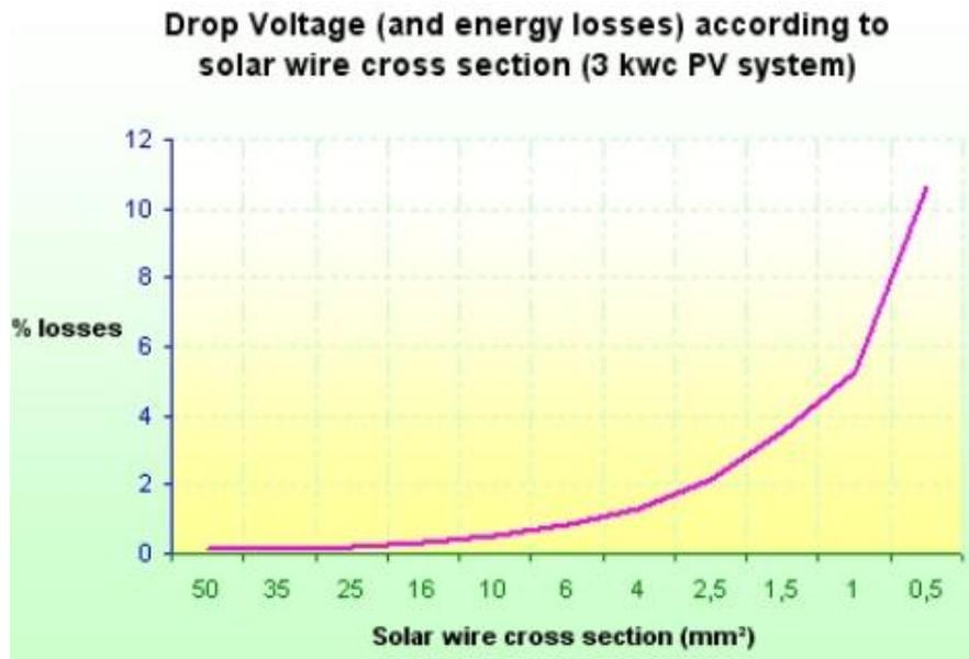
FIG. 4. Voltage drop losses according to wire cross section for a PV system of 3 kWp with 50 m of solar DC string cable.
