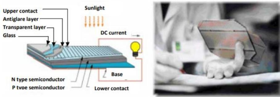
**FIG. 1.** Typical monocrystalline cells
