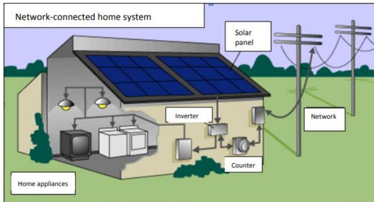
**FIG. 2.** Network-connected photovoltaic system
