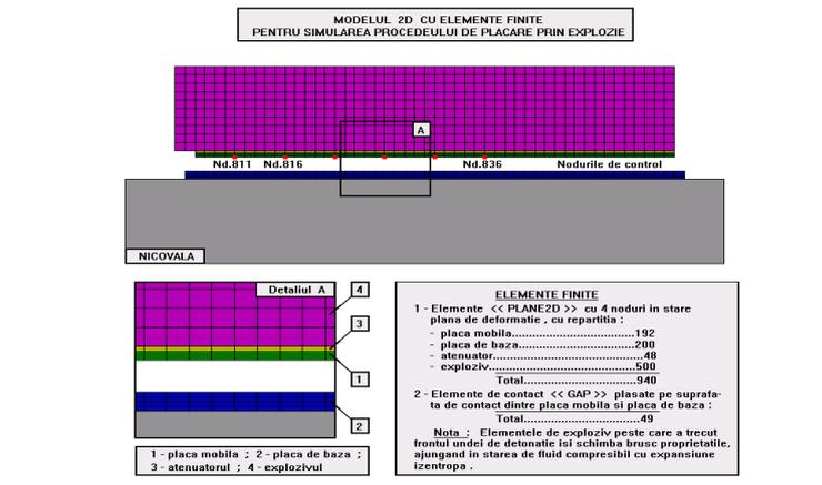
**FIG. 1.** The 2D Finite Element Model from the simulated Explosion Welding Process.
