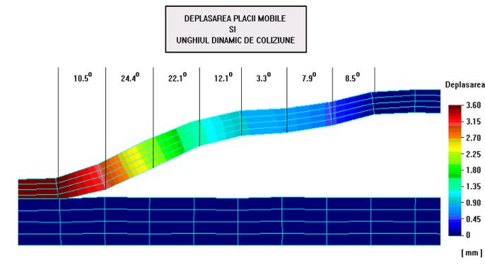
**FIG. 4.** The mobile plate moving and the dynamic angle collision.
