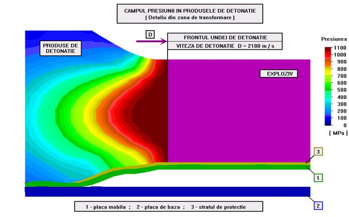
**FIG. 5.** Pressure field in detonation products: D - the detonation wave front; 1- the movable plate; 2- the basic plate; 3- the protect layer.
