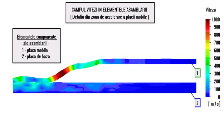
**FIG. 3.** The speed's field in the assembly elements: 1- the movable plate; 2- the basic plate.
