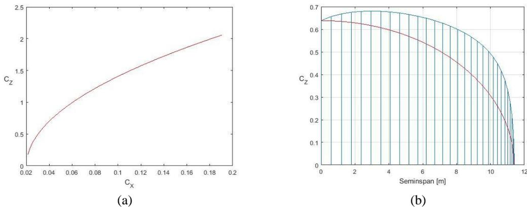
FIG. 3. Code validation (a) Lift-Drag distribution, (b), Lift distribution over the wing
