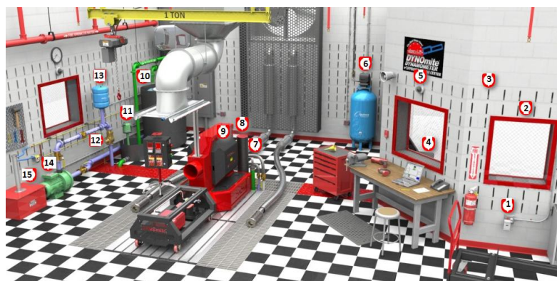
FIG. 3. The typical engine dynamometer test cell
