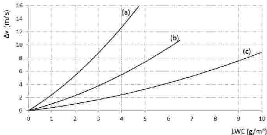
**FIG. 2.** Difference in velocity of wet and dry airstreams versus liquid water content at temperature 24 °C for airflow velocities: (a) 11 m/s, (b) 8 m/s, (c) 5 m/s
