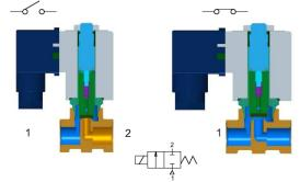
Fig. 1. Direct acting solenoid valve [3]
