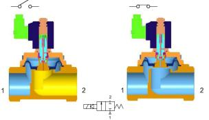
Fig. 3. Indirect operated solenoid valve with forced lifting [3]
