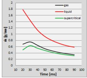
Fig. 11. Discharging mass flow rate
