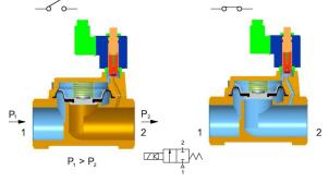
Fig. 2. Pilot operated solenoid valve [3]
