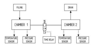
Fig. 8. Block schematic diagram
