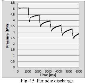
Here, the solenoid control valve opens periodically for 50 ms at intervals of 1 second. The periodic discharge flow to the surrounding atmosphere was stabilized by using the orifice of diameter 1.6 mm that was placed behind the control valve. The initial liquid  $CO_2$  filling was 70 g.
