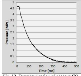
Fig. 12. Depressurization of gaseous CO<sub>2</sub>
