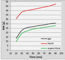
Fig. 10. Valve discharge characteristics
