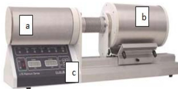
Figure 7. General Presentation: a) dilatometer measurement system; b) furnace; c) command and control system;
