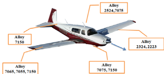
Figure 1. Highlighting construction aluminium alloy features from a commercial aircraft [2].
