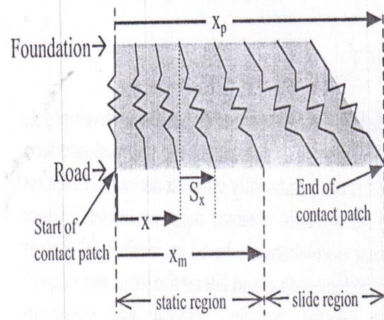
Fig. 2 “Brush” Analog used to Describe Longitudinal Tire Behavior along Tire Contact Patch
