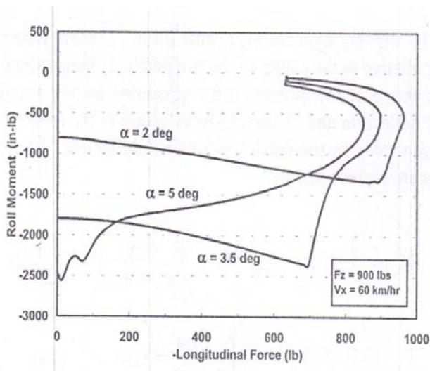
Figure 10 Roll moment predictions-dry pavement
