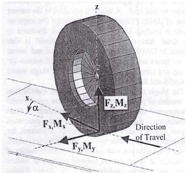
Fig. 1 Calculated Tire Forces and Moments [1].
