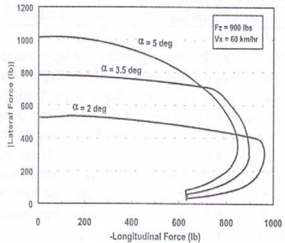
Fig. 8 Tire force prediction-dry pavement
