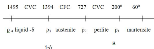
Figure 1. The cooling structure diagram of the steel
