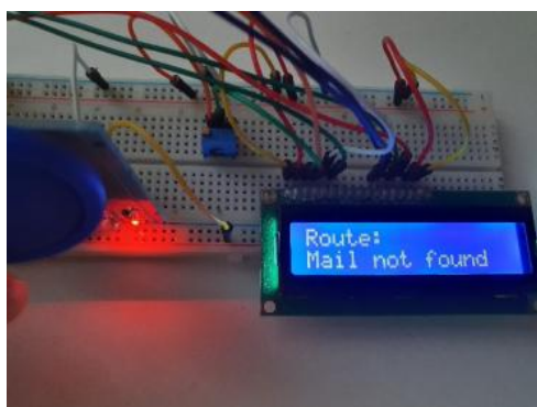
Fig.12 The result of scanning the unidentified RFID tag in main sorting center
