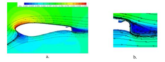
**FIG. 14.** a) Flowfield around DU97 flatback airfoil ( $V_{\infty} = 30 \text{ m/s}$ , incidence angle =  $15^{0}$ , Re= $3.0 \times 10^{6}$ , C<sub>u</sub>=0.030); b) detail of TE flowfield
