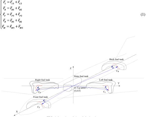
FIG. 1 Location of aircraft fuel tanks
