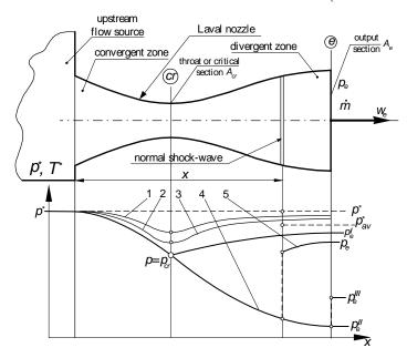
FIG. 2 Laval-type exhaust nozzle starting process [8]
