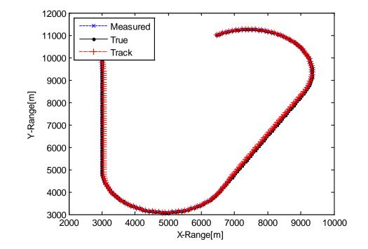
On the opposite, the second Kalman filter can accurately track the maneuver (Fig.7), but the estimated error at constant velocity is greater (Fig.8).
