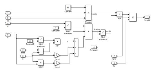
FIG. 6 K<sub>x</sub> Matlab/Simulink block diagram
