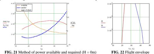
Doing the same for all altitudes for which the outputs for the shaft power supplied by the engine are calculated: 1000, 2000 and 3000m, it can be obtained V2(H) and V1(H), which are graphically represented in the flight envelope of Fig. 22.
