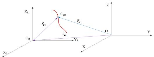
FIG. 2 Center of gravity's position vector for a fuel tank (the right wing tank)
