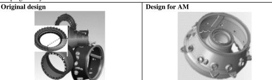
**Design features:** Original design features include mechanical assembly function from circumferential holes and bosses as well as flanges in aft and forward sides. The design intent comprises of structural integrity at elevated temperatures.
