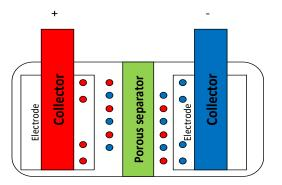
FIG. 1. The internal structure of a super capacitor
