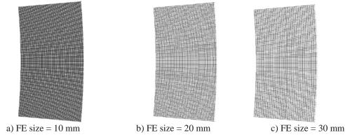
FIG. 5 Finite element models
