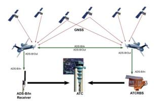
FIG.6. ADS-B transmission, [14]
