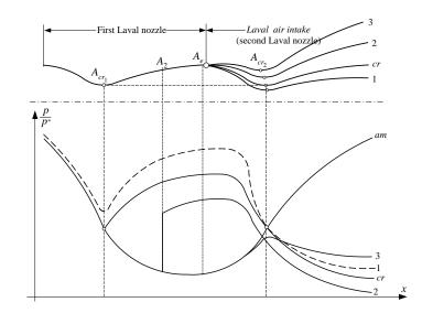
FIG. 3. Laval-type air intake starting process [8]
