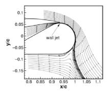
FIG. 1. Circulation control around a curved trailing edge of an airfoil.
