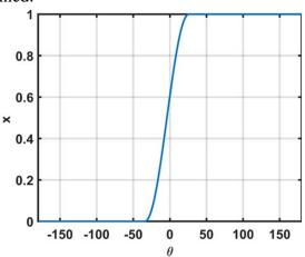
**FIG. 6** The variation of the burning mass fraction burned with the crankshaft angle.
