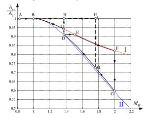
FIG. 5 Laval-type air intake work lines used as control law(s)
