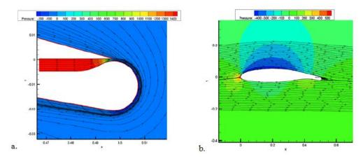
**FIG. 8.** Streamlines and pressures field: (a) without external flow  $(V_{jet} = 9 m/s, V_{\infty} = 0 m/s)$  and (b) external flow without jet  $(V_{\infty} = 30 m/s)$
