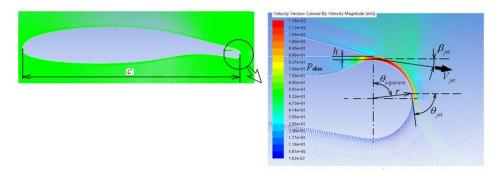
FIG. 3. Geometric data on the rounded trailing edge for the Coanda type flow
