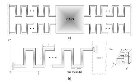
FIG. 2 Serpentine schematic representation: a) overall configuration with four springs; b) one typical spring
