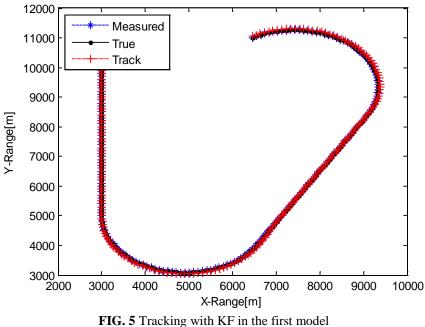
The first Kalman filter tracks the course at a constant velocity (Fig. 5), the calculated error is insignificant, but when it tracks the maneuver, the calculated error becomes tangible - about 40 meters (Fig. 6).
