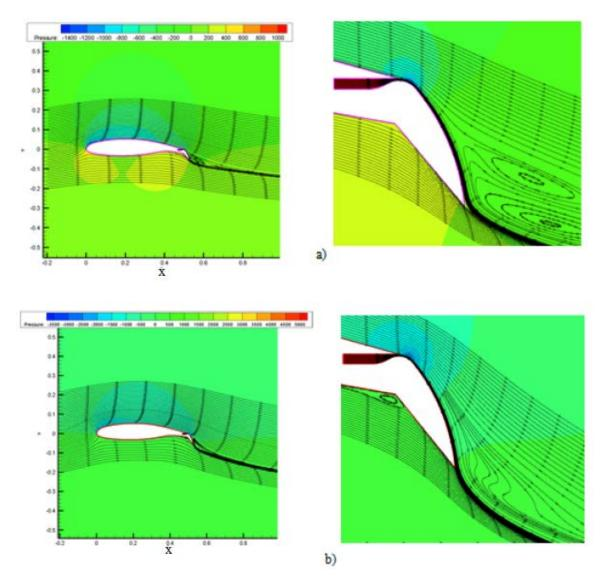
**FIG. 12.** Flowfield (streamlines and pressures) for two numerical simulations cases, with details: (a)  $V_{jet} = 10.55 \text{ m/s}$ ;  $V_{\infty} = 30 \text{ m/s}$ ; (b)  $V_{jet} = 20 \text{ m/s}$ ;  $V_{\infty} = 30 \text{ m/s}$
