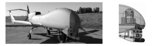
FIG.4. UAV with sense and avoid detection system, [6, 7]
