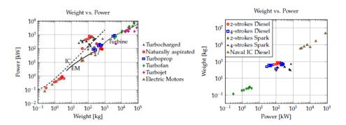
FIG. 1 Power-weight correlation for various engines. [5]
