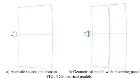
The authors have opted for a 2D axisymmetric model, this being most convenient (easy to build, shorter computer time).
