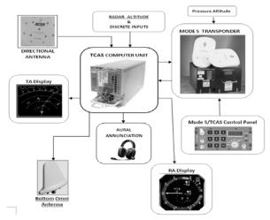
FIG.2. Simplified block scheme of the TCAS system [1].
