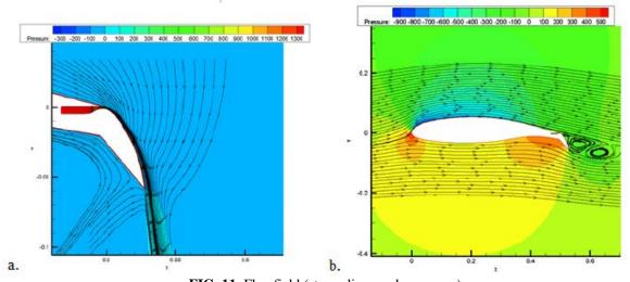
**FIG. 11.** Flowfield (streamlines and pressures): (a) without external flow ( $V_{jet} = 9m/s$ ;  $V_{\infty} = 0m/s$ ) and (b) external flow without jet ( $V_{\infty} = 30m/s$ )
