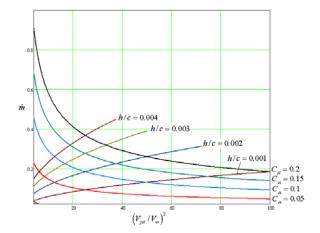
FIG. 5. Required mass flow rate for circulation control
