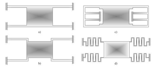
**FIG. 1.** Elastic structures for inertial sensors: a) fixed-fixed flexure; b) crab leg flexure; c) folded flexure; d) serpentine flexure
