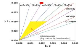
FIG. 6. Optimum geometry domain of the most effective circulation control
