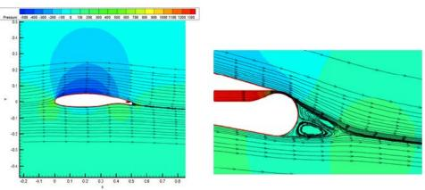
**FIG. 9.** Streamlines and pressures field with TE details;  $V_{jet} = 9 m/s$ ,  $V_{\infty} = 30 m/s$
