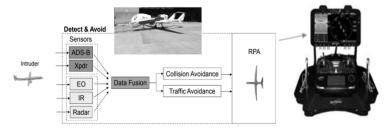
FIG.5. Sense and avoid system operating diagram [7].
