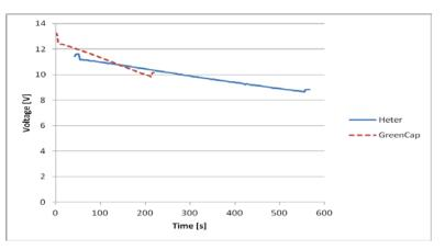
FIG. 5. Voltage evolution at super-capacitor battery terminals
