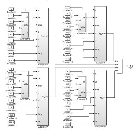
FIG. 3 Matlab/Simulink model for the serpentine flexure
