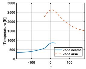
FIG. 7. Temperature variation in the burned and unburned area with the crank angle.
