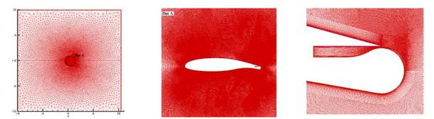
FIG. 7. Computational domain, meshing and trailing edge details
