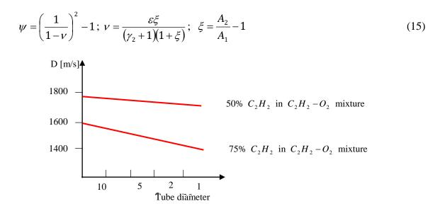
FIG. 2 The dependency of the detonation velocity on the tube diameter
