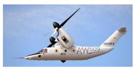
FIG. 6 Tilt rotor vectored thrust
