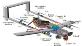
FIG. 25 The power system of the uav - biplane-quad-copter hybrid
