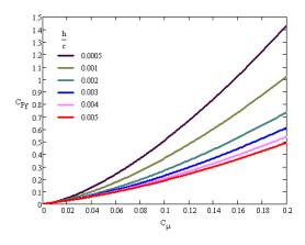
**FIG.4.** Required coefficient fluid power for "Coandă" type jets, for various h/c ratios
