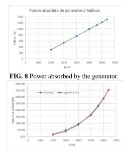
FIG. 9 Simulation comparison and SLS experiment for engine 3w 55xi fi.
