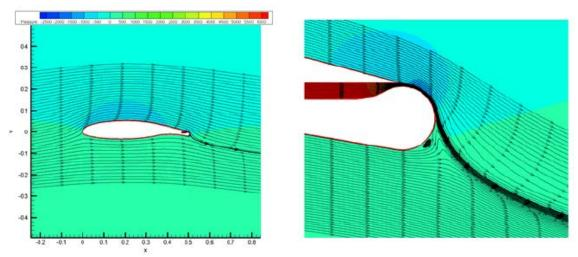
FIG. 10. Streamlines and pressures field with TE details;  $V_{jet} = 20 m/s$ ,  $V_{\infty} = 30 m/s$
