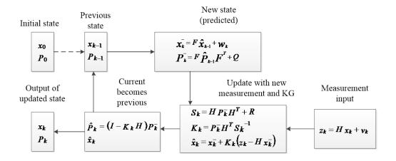
FIG. 1 A complete picture of Kalman filter operations
