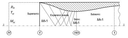
FIG. 1 Supersonic inlet with internal compression of inverted Laval type
