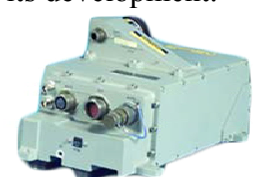
Elektronic unit (WRA-2) of system AN/AAS-52 (MTS)
