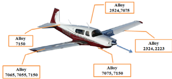
Figure 1. Highlighting construction aluminium alloy features from a commercial aircraft [2].
