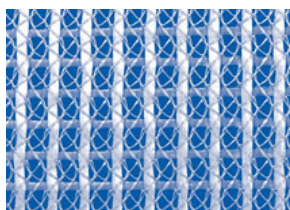
Figure 2. Illustration of a stitch-bonded fabric
