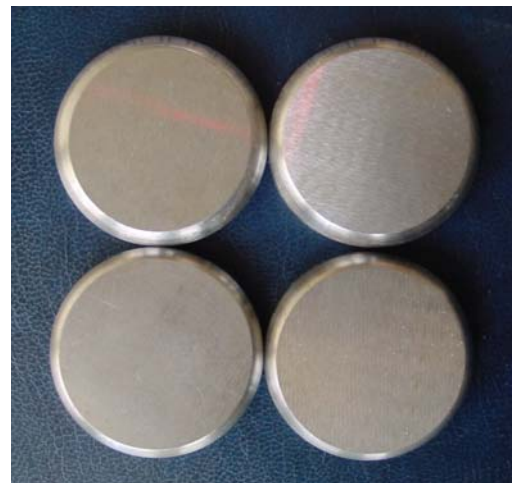
Fig.2. The mobile semi coupling (steel OLC 45)
