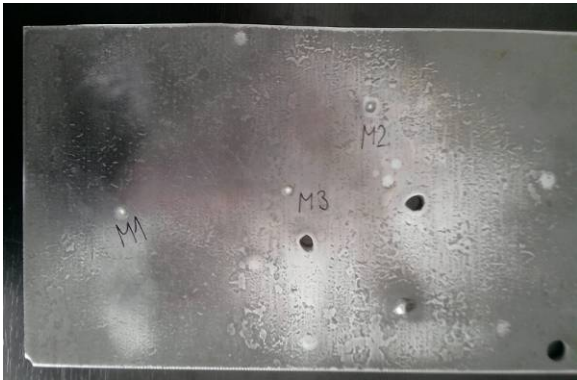
Fig. 5: Location of the chemical analysis (M1, M2, M3)
