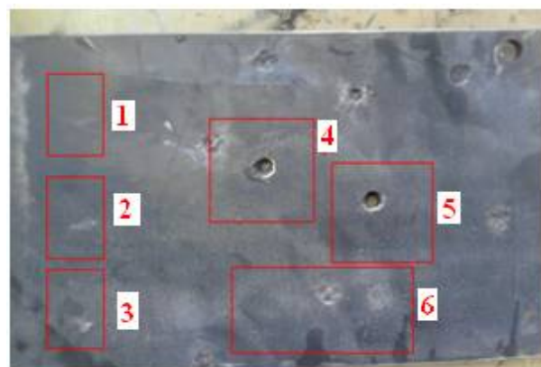
Fig. 4: Areas of hardness measurements on a sample
