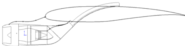
Fig. 1. Proposed way to integrate a CELTIS system using a high by-pass turbofan engine within a supercritical wing
