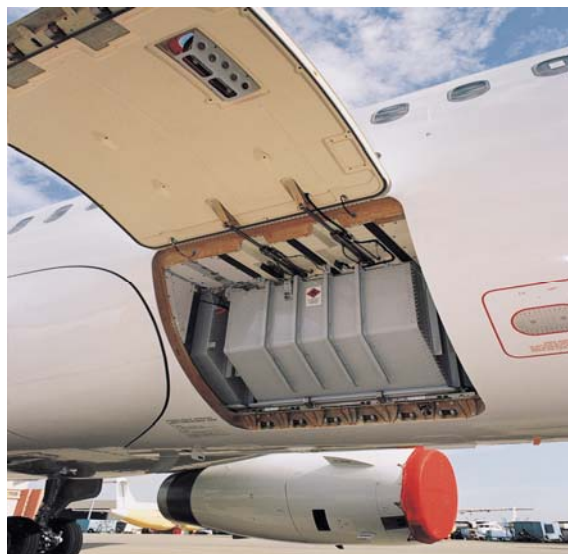
Fig. 3 Installation of additional fuel tanks in the freight hold
