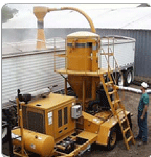
Fig. 2.4. b. Self-powered super suction
