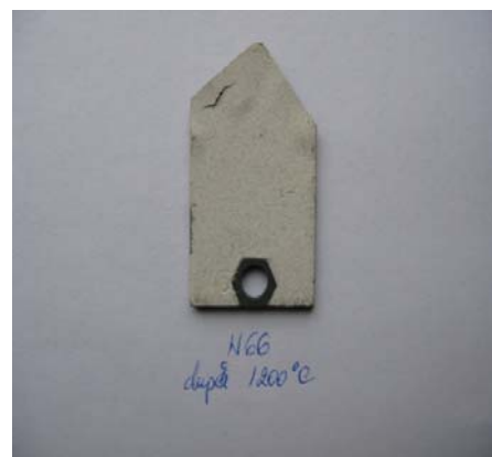
Fig.6. shows surface cracks of N66, deposit NiCr/ ZrO 2 Y 2 O 3
