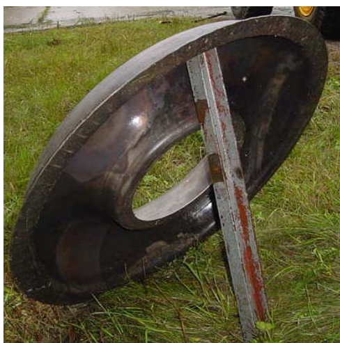
Fig. 7. Piece drawn by explosive forming
