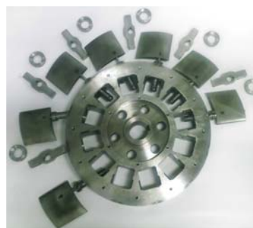
Fig. 1 – Turbine with partially set-up blades( axis blades, clinches and balancing counter-weights)
