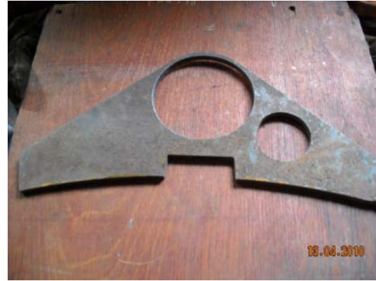
Fig. 5. Part plasma cutting
