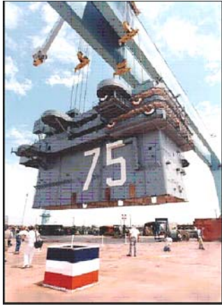
Figure 4. Special crane used in ship block material handling
