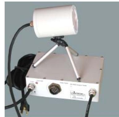
Figure 4. BR/1502 Doppler radar fitted with an aerial
