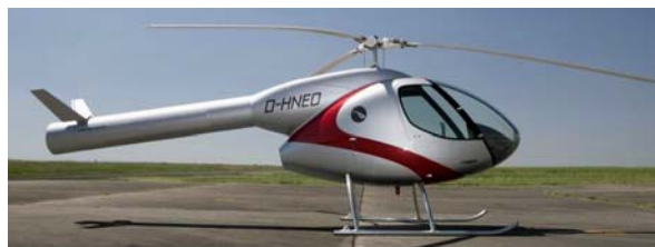
Fig. 5. The NOTAR system used by NEO helicopter from YoungCopter
