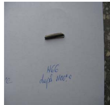
Fig.5. N66 sample for microscopic investigations after quick thermal shock test at 1100 ° C
