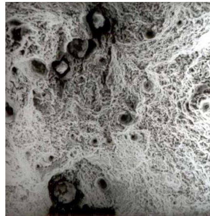
Fig. 6 Typical folds of ESR forgings
