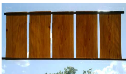
Fig. 2 Experimental trial stand for sunlight exposure
