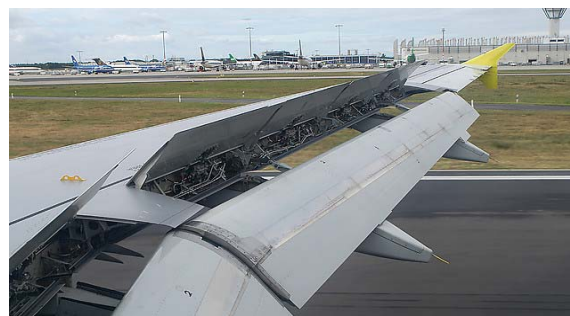
Fig. 4 Wing mechanization of the A319CJ airplane
