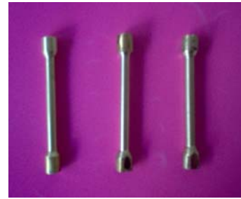
Fig.4. Standard samples, from memory shape alloys type CuZnAl, for thermal fatigue test.
