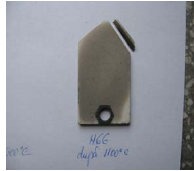
Fig.4. N66 specimen on Nimonic 80 support / deposit NiCr/ ZrO 2 Y 2 O 3 after quick thermal test shock at 1100 ° C
