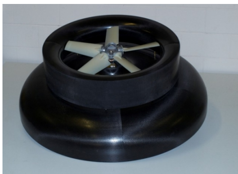
Fig. 13 ODIN – The AESIR's demonstrator for a military Coandă UAV
