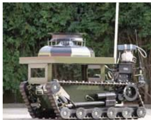
Fig. 16 EMBLA - in its counter IED role on top of a Northrop Grumman Remotec Mk 8 EOD Wheelbarrow
