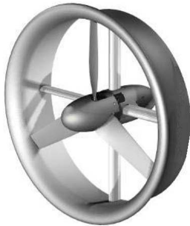
Fig.5. Constructive solution with stator.
