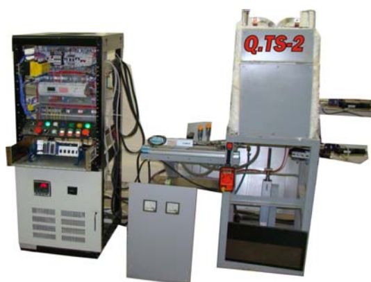
Fig.11. Installation for material testing in extreme heat conditions
