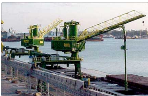
Fig.2.8 SuperTower@ Model 405/22.5 Fanless Shipunloaders
