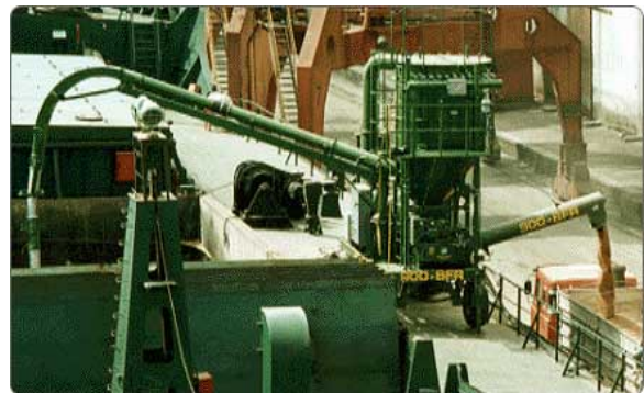
Fig.2.10 SuperPortable discharging ship in Brazil
