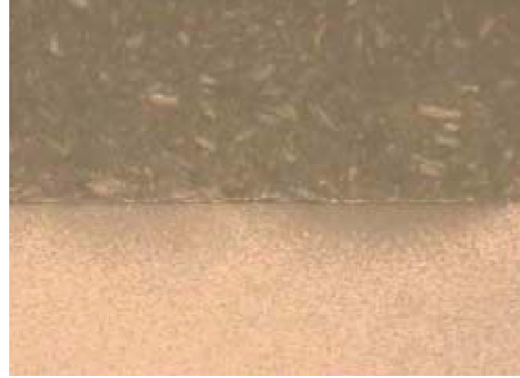
Fig. 8. Photomicrograph of a cross section of hardness zone. Max. hardness is 47HRC and at a case depth of 0.5 mm is 41HRC.
