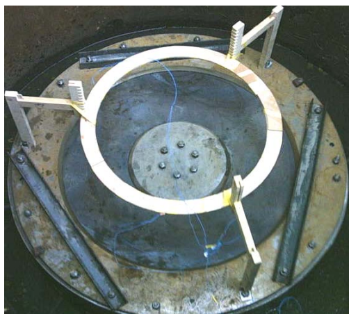
Fig. 6. Die ready for underwater explosion
