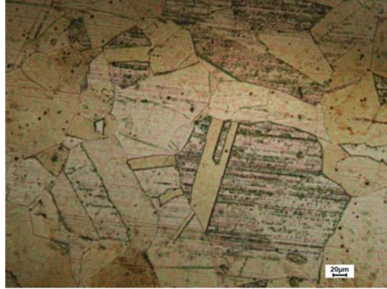
FIG.4 X5CrNi18-10. Metallographic structure after solution immersion quenching from 1050°C and artificial ageing at 510°C. Aqua regia etching. 1000:1
