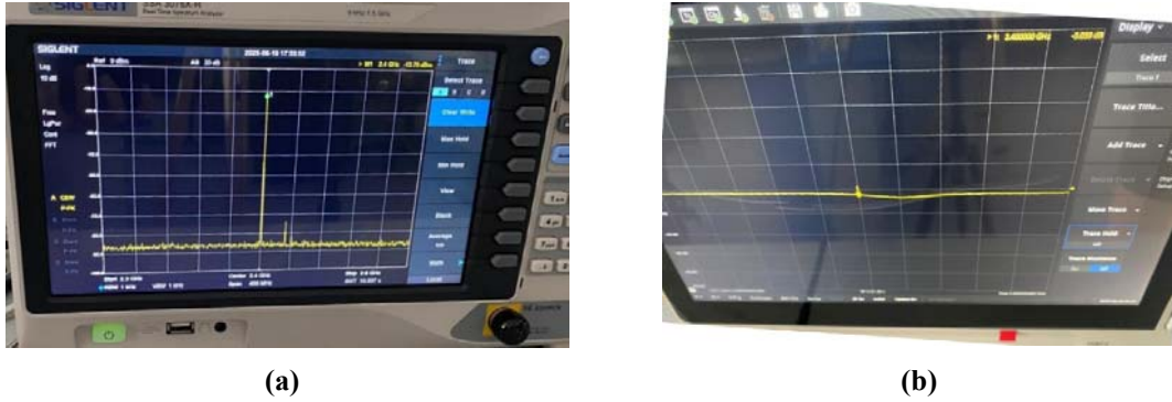
FIG.7 Resonant frequency obtained on the spectrum analyzer [4]. (a) Signal reception with the patch antenna at 2.4 GHz. (b) Reflection coefficient
