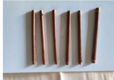
**FIG. 7** Final copper anode segments
