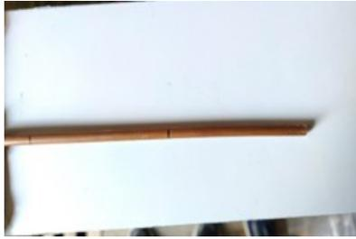
**FIG. 6** Marking the copper tube for cutting
