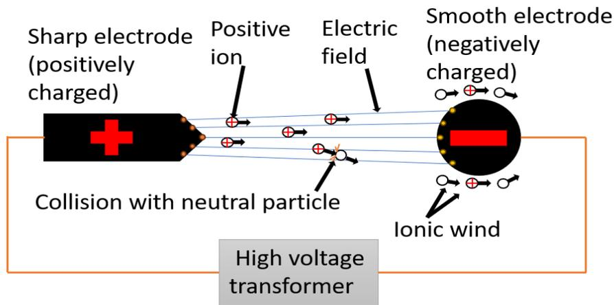
FIG. 1 Schematic representation of the electric propulsion phenomenon
