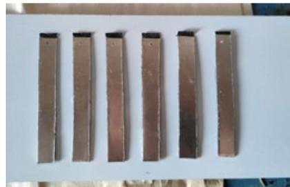
**FIG. 9** Completed set of six aluminum cathodes
