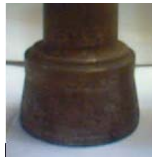
Fig. 4: Punch loaded by welding
