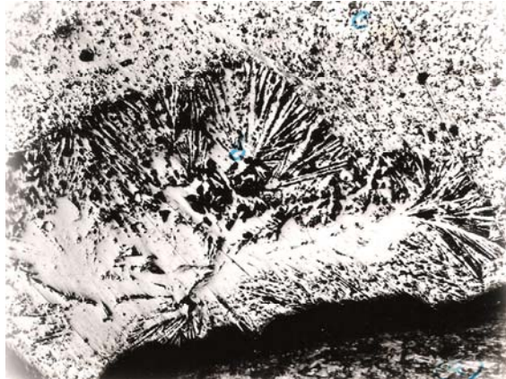
Fig. 6. Fused and solidified metal in Cu flyer plate near interface
