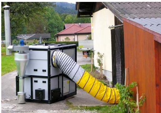
Fig. 5 – Heating of buildings with a biomass (wood chips) mobile air unit
