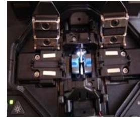
Figure 5 - guiding mechanism, welding equipment and electrodes microcamerele fiber
