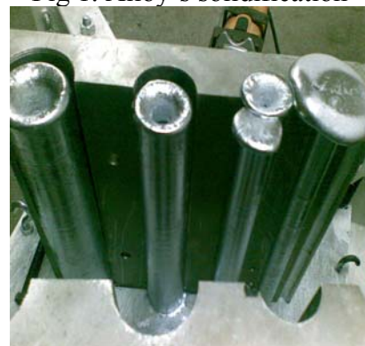
Fig. 2 Extraction of vibrated samples from the mold
