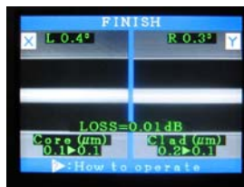
Fig. 12 - Measuring the attenuation
