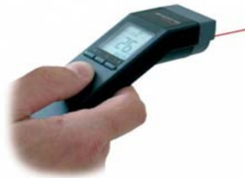
Figure 4 The pyrometers Micronics OS 524 E type
