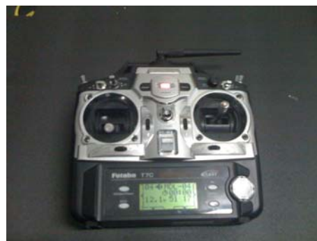
Fig.6 Remote control used for controlling the aeromodel
