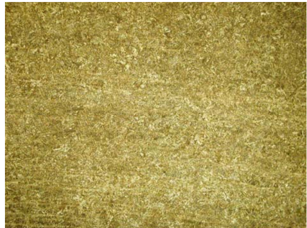
Fig. 4 Microstructure of base material (ARMOX 500), 500x
