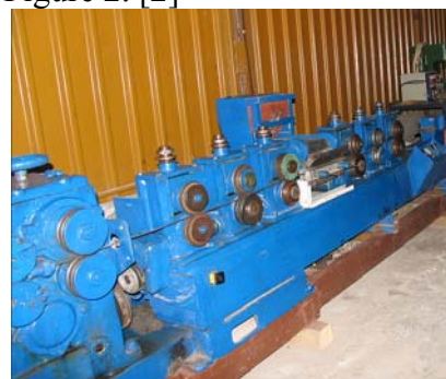
Fig. 2: Tubular rods production line
