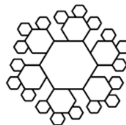
Fig. 1. The architecture of the fractal antenna with hexagonal resonators.
