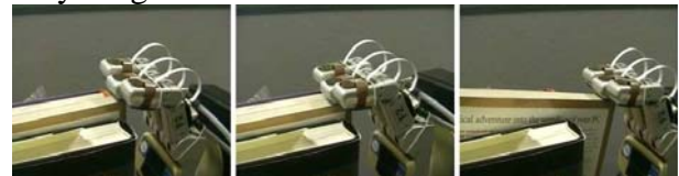
Fig. 3. The robot grasping the book. Left: initial contact. Middle: Maximizing contact surface. Right: doing the task. (A. Morales et al., 2007)
