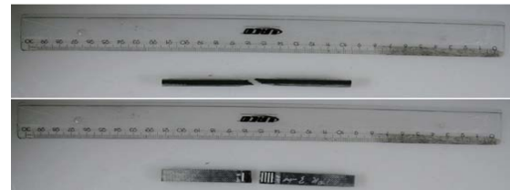
Fig.7: The most common fracture pattern of specimens for \pm 45^\circ fibers orientation
