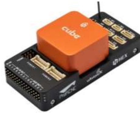
FIG. 9 Cube Orange with Pixhawk motherboard
