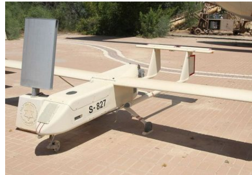
FIG. 2.7. Tadiran Electronic Systems Mastiff , [15]
