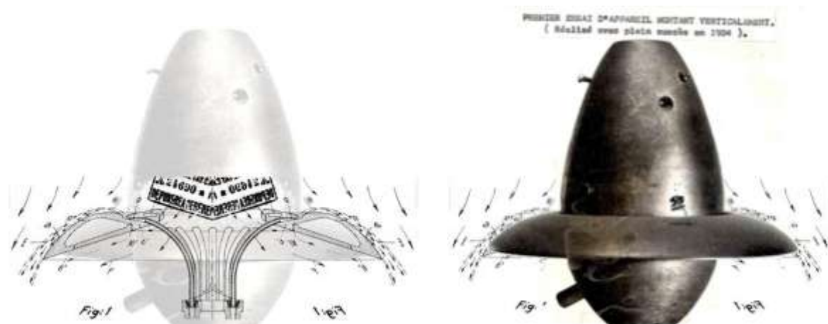
FIG.3 The Coanda Effect thruster successfully tested in 1932
