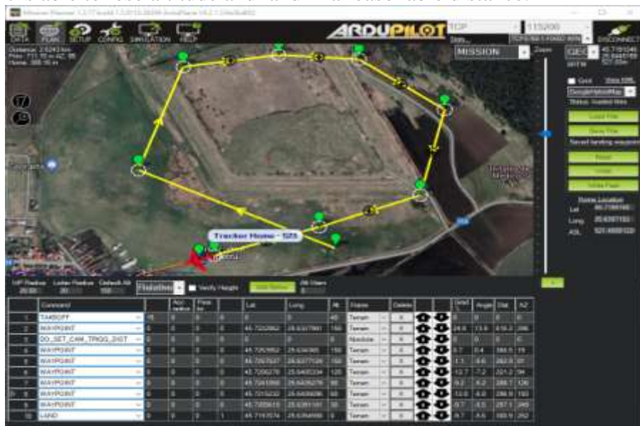
FIG. 5 Landing path generated in Mission planner
