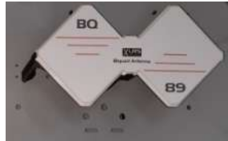
FIG. 5 The Smart Antennas SMBTS (Smart Base Station) front view
