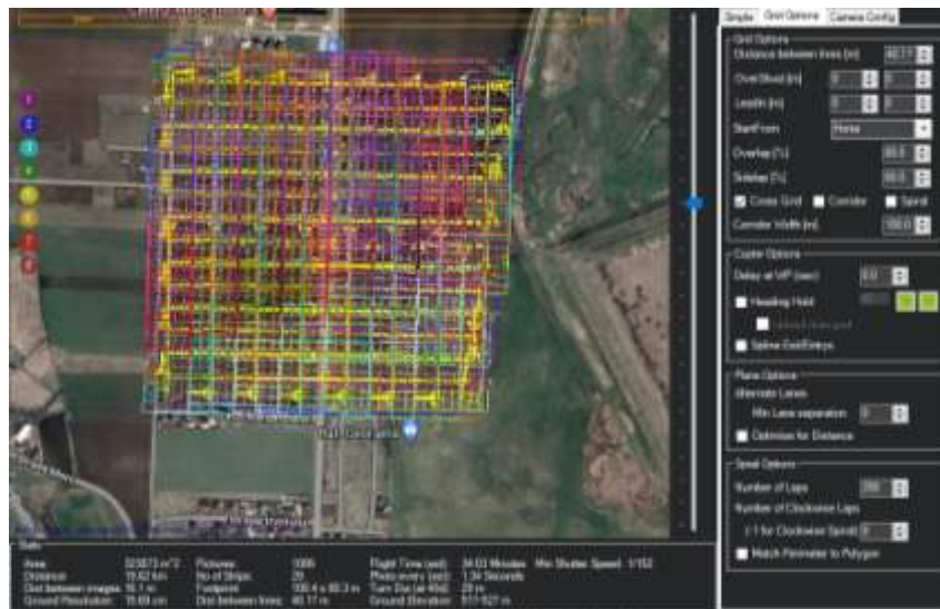
FIG. 6 Survey grid with picture squares simulation overlap
