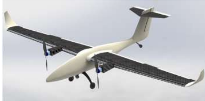
FIG. 1 Simulation of the model aircraft made from 3D printed composite materials [10]
